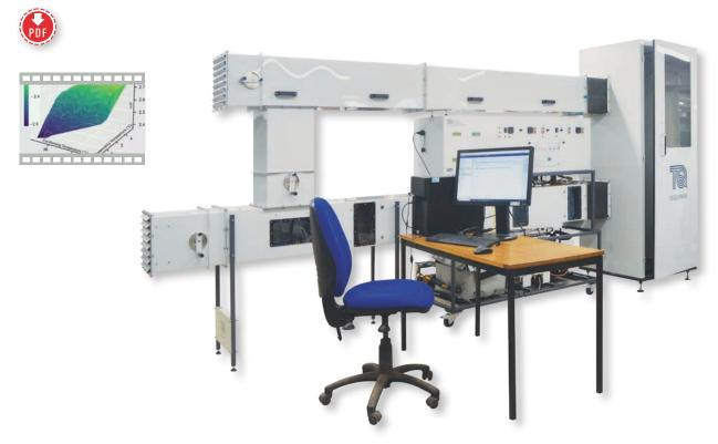
BASE UNIT (ECI55OV) FITTED WITH THE OPTIONAL RECIRCULATION DUCT AND ENVIRONMENTAL CHAMBER
