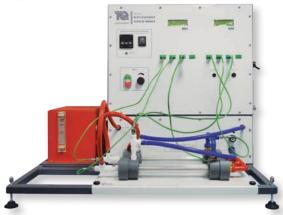
SERVICE MODULE FITTED WITH THE CONCENTRIC TUBE HEAT EXCHANGER EXPERIMENT (TD1360A)
