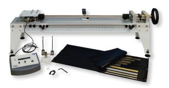
Benchtop apparatus tests different types of struts and demonstrates how they deflect under load, and demonstrates the use of Southwell's method. Set of additional struts available.
