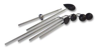
A set of different shape models with identical frontal area to allow students to compare the different coefficient of drag for each shape. Includes a dummy stem for tests to cancel out the drag due to each model's support arm. Note: You also need the optional two or three component balance (AF1300z or AF1300t) for direct readings of drag.
