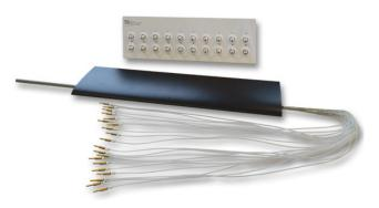
The aerofoil has 20 static pressure tappings along its chord on the upper and lower surfaces. They each connect to tubes that pass through the aerofoil and then out to clear, numbered, flexible tubes. Students can connect the tubes to other optional pressure-measurement instruments. They can then measure the pressure distribution around the aerofoil, from which they can find the lift.
