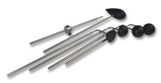
These models fit into the working section. They are held by the balance and allow students to see how shape affects aerodynamic drag. The models include 'classic' aerodynamic test shapes including a smooth sphere, a dimpled sphere and a streamline shape.
