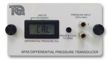
and other pressure-sensing devices fitted to a wind tunnel, with respect to the atmosphere or differential pressures.
