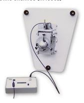
This simple to fit balance mounts onto the side of the wind tunnel working section. The balance works with both the supplied and other optional models.
