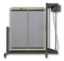
A 36-tube tilting manometer for measuring pressure in subsonic wind tunnels, including TecQuipment's AF1300. A backboard with a graduated scale holds each manometer tube.
