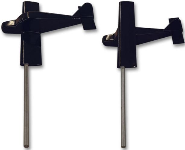
Model aircraft with NACA profile wings. One has a low wing position (bottom of the fuselage), the other has a high wing position (above the fuselage). These models are good for experiments with lift, drag and pitching moment of fixed wing aircraft.
