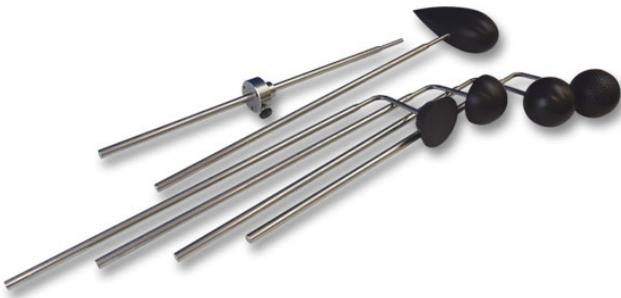
A set of different shape models with identical frontal area to allow students to compare the different coefficient of drag for each shape. Includes a dummy stem for tests to cancel out the drag due to each model's support arm.
