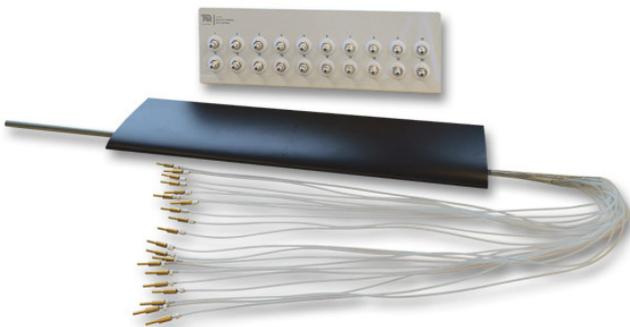
The aerofoil has 20 static pressure tapings along its chord on the upper and lower surfaces. They each connect to tubes that pass through the aerofoil and then out to clear, numbered, flexible tubes. Students can connect the tubes to other optional pressure-measurement instruments. They can then measure the pressure distribution around the aerofoil, from which they can find the lift.
