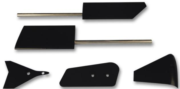
A pair of two wings, one incorporating a raked winglet, enabling students to explore three dimensional wing theory.
