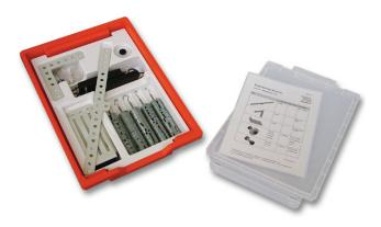
The rigid beam allows experiments that show the use of moments to find unknown weights, creating simple beam balances. It also works with spring balances to show reaction forces on beams with point loads and uniformly distributed loads (UDLs).
