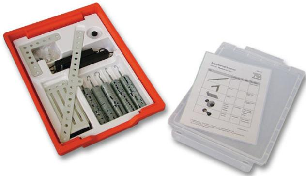
The rigid beam allows experiments that show the use of moments to find unknown weights, creating simple beam balances. It also works with spring balances to show reaction forces on beams with point loads and uniformly distributed loads (UDLs).
