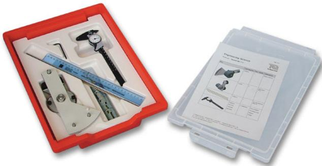
Standard tests show the relationship between torsion and 'J' (polar second moment of area) value. Students use this to predict the twist angle for any given specimen.
