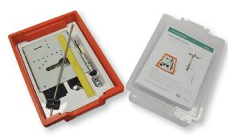
The theory shows how to predict the period of oscillation for a given pendulum or spring for comparison with actual results. The kit includes an experiment with the Kater's pendulum that shows the relationship between simple harmonic motion and gravity, for prediction of gravity to a reasonable accuracy.
