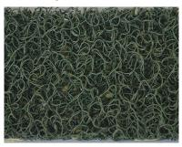
A roughened bed section to allow students to determine and compare the losses in a smooth flow channel with those experienced in a channel with a roughened surface.
