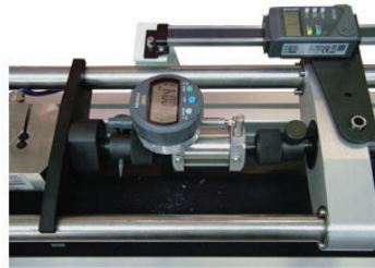
OPTIONAL EXTENSOMETER (SM1002A) FITTED TO TL SPECIMEN
