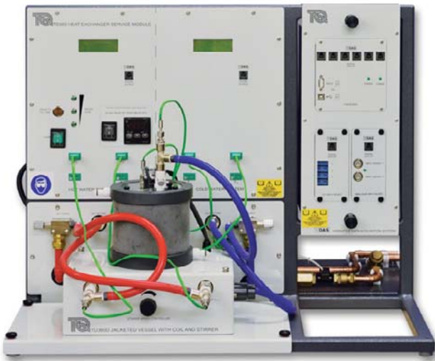
THE SERVICE MODULE (TD360) SHOWN WITH THE JACKETED VESSEL WITH COIL AND STIRRER HEAT EXCHANGER MODULE AND THE OPTIONAL VDAS® UNIT (VDAS-F)
