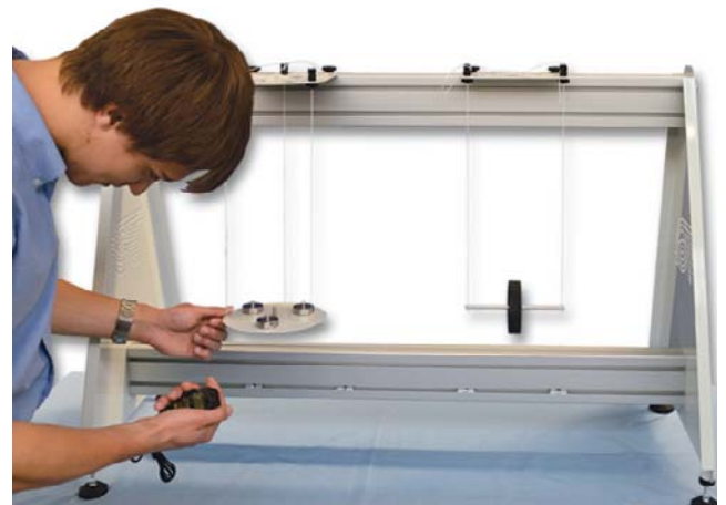
THE FILAR PENDULUMS MODULE IN USE, SHOWN FITTED TO THE TEST FRAME (TM160)
