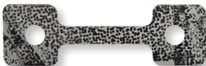
SPECIMEN WITH APPLIED SPECKLED PATTERN
