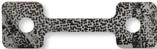
SPECIMEN WITH APPLIED SPECKLED PATTERN
