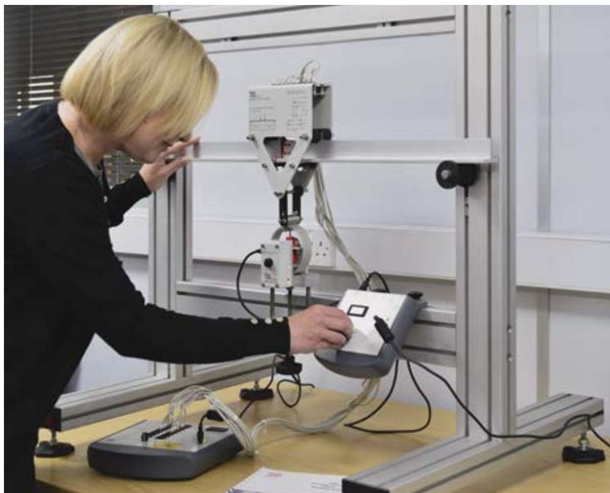
TEST FRAME (STRI) FITTED WITH THE EXPERIMENT MODULE BENDING STRESS IN A BEAM (STR5) AND DIGITAL FORCE DISPLAY (STRIA)
