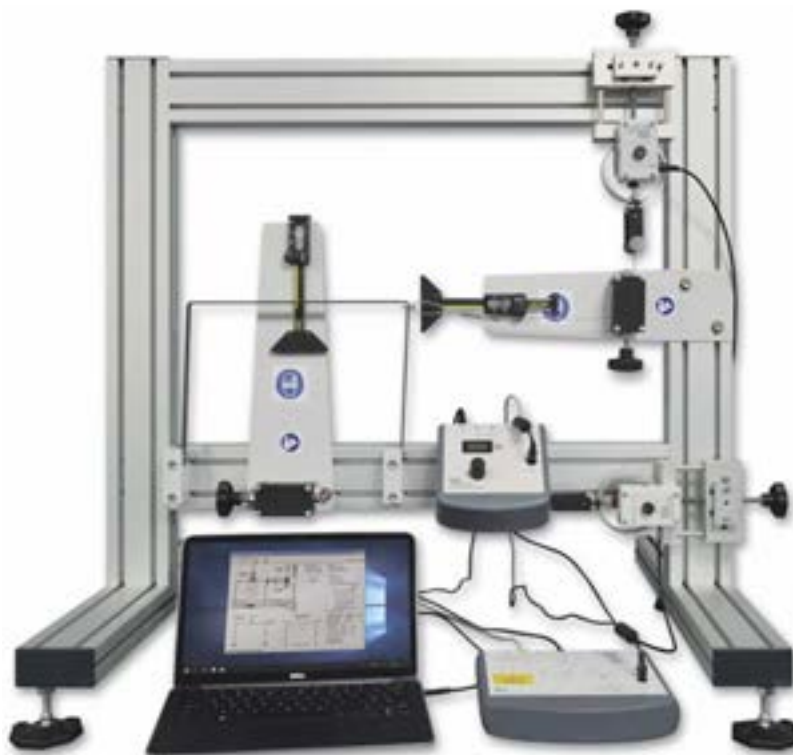
THE STR2000 COMPUTER INTERFACE UNIT SENDING DATA FROM ONE OF THE STRUCTURES HARDWARE EXPERIMENT MODULES TO THE STRUCTURES SOFTWARE
