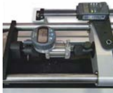
OPTIONAL EXTENSOMETER (SM1002A) FITTED TO TL SPECIMEN
