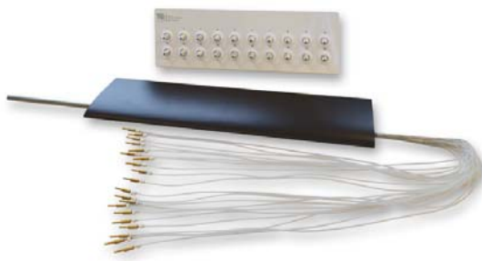
NACA 0012 AEROFOIL WITH TAPPINGS AFI300B
